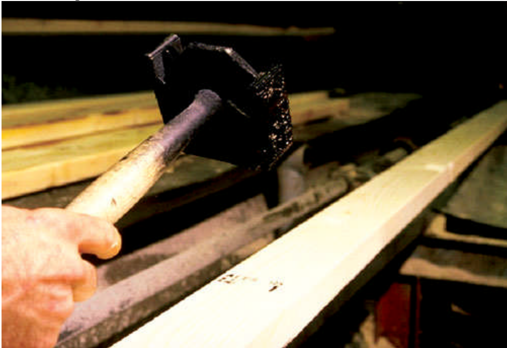
A grade stamp is put on every piece of lumber for use in Canada and the U.S.
